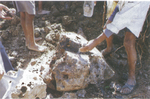
Fig. 3. View of a test pit showing a block of rhyolite with opal nodules.
