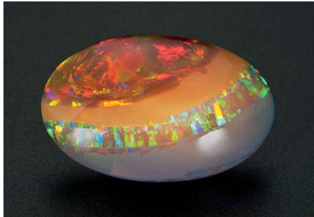
Figure 10. The strong zoning of this exceptional 18.68 ct cabochon represents most of the opal varieties found at Wegel Tena: brownish orange to white, transparent to opaque, with and without play-of-color. The zoning probably corresponds to successive deposition of horizontal opal layers in a cavity. The white layer with strong play-of-color shows parallel columns that we refer to as digit patterns. Note that they are perpendicular to the plane of zoning, which means they developed vertically. Photo by Robert Weldon.
