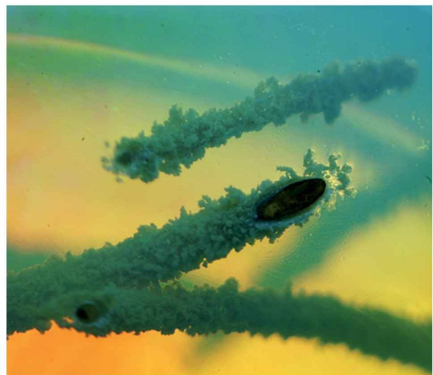
Figure 17. Elongated, cylindrical inclusions were present in one opal sample. This coated cylinder was made of silica, most likely chalcedony. Photomicrograph by B. Rondeau; magnified 40 \times .
