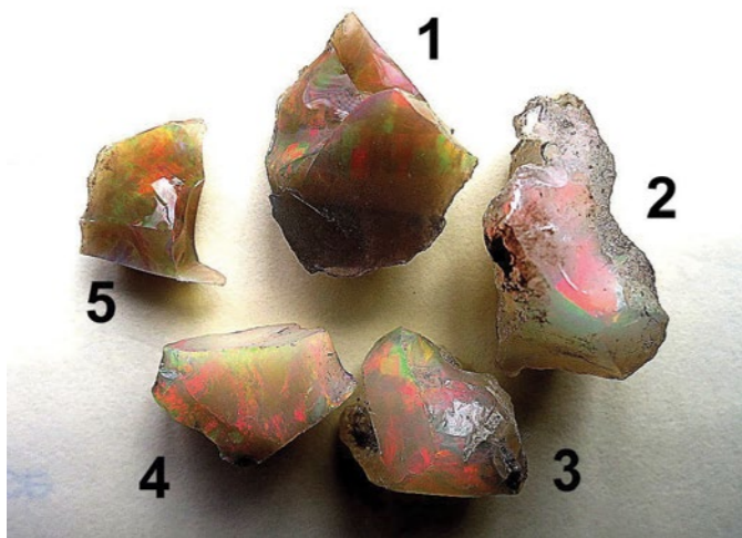
Figure 2. Ethiopian Welo opal fragments with POC, used for porosity testing.
