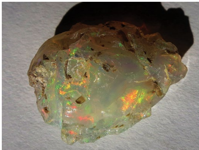
Figure 24. Welo "Crystal-ABR" specimen, showing the surface-reaching cavity-perforations that could retain water during its nominal surface removal, and which then reports as an erroneous excessive voidage. Specimen is about 15 mm across.
