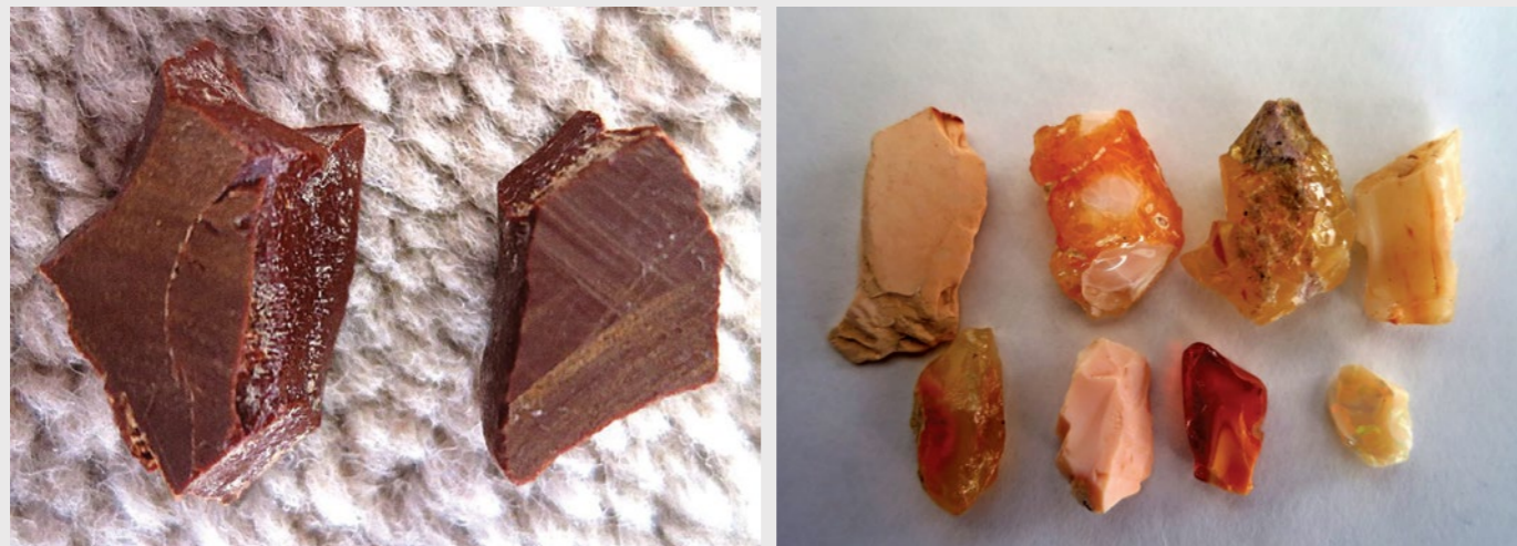
Figure 21a and b. Left: Dual portions of Shewa "magnetic" opaque patch hydrophane, as in Figures 16 and 17, used for porosity determination. Discontinuities displayed on the exposed glossy fracture surface reflect the presence of numerous magnetite cubic pseudomorphs after pyrite (see also Figure 17).
