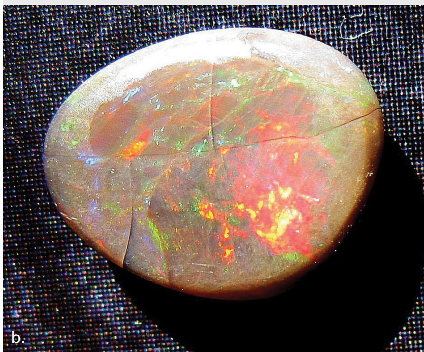
Figure 20a and b. Javanese opal specimens immersed in water for their voidage determination, causing one to instantly fracture into several fragments, presumably due to differential peripheral hydration-expansion and consequent stress development.
