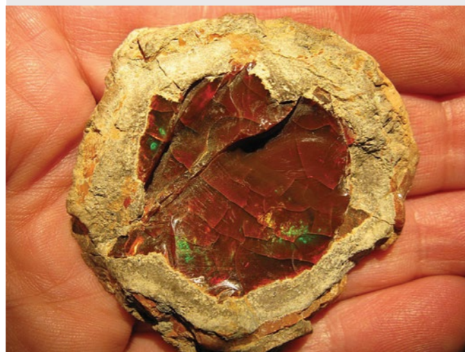
Figure 3. Ethiopian Shewa gem-opal nodule, naturally-fractured due to intrinsic internal stress.
