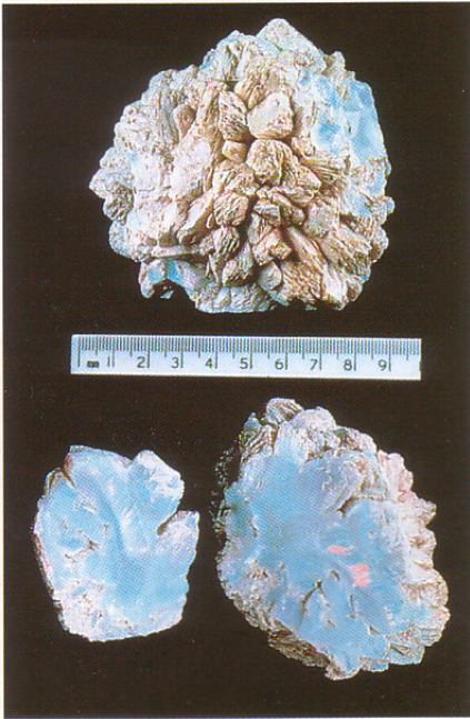
Fig. 1 White Cliffs opal 'pineapples'. Opal pseudomorphs after the mineral ikaite. (Australian Museum photograph)
